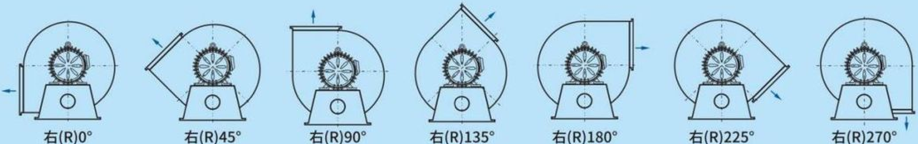
右旋:从电机端或传动组端正视顺时针方向旋转 Right-rotated: Watching the motor by side the impellers rotate clockwise
