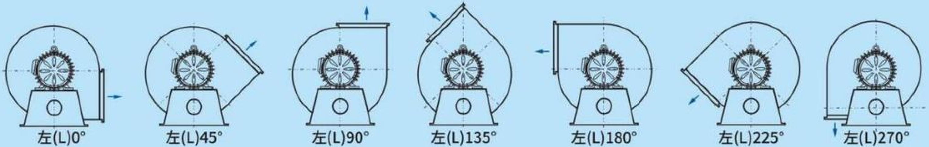
左旋：从电机端或传动组端正视逆时针方向旋转 Left-rotated: Watching the motor by side the impellers rotate anti-clockwise
